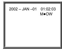
NOTE: If the HDDs' capacity is only 5 GB left, it will buzz for 3 seconds; so as in 4GB, 3GB, 2GB and 1GB. If the O/W Recording mode(NOTE 1) is on, it won't have the warning buzzer.
